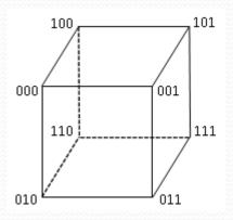
On a hypercube, the shift operator maps the state  $|k,v\rangle$  into  $|k,v_j\rangle$ , where the n-bit strings v and  $v_j$  differ by the j-th bit. So, the shift operator S can be represented as follows
