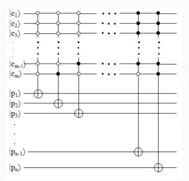
where  $|c_1\rangle|c_2\rangle...|c_m\rangle$  is the coin state and  $|p_1\rangle|p_2\rangle...|p_n\rangle$  the position state (the vertex state).
