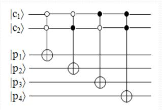
The first gate flips the target qubit if and only if the control qubits are set to o.
