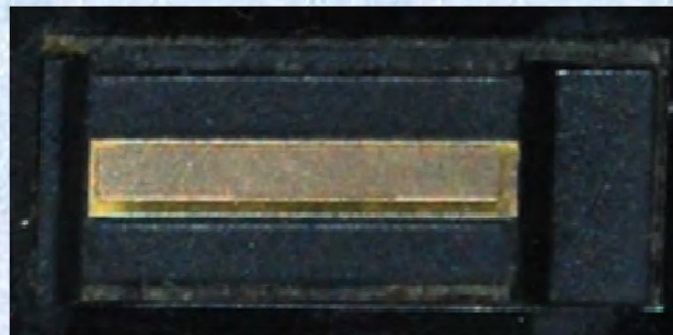
Mouse with a sweep fingerprint sensor and the detail of the sensor
