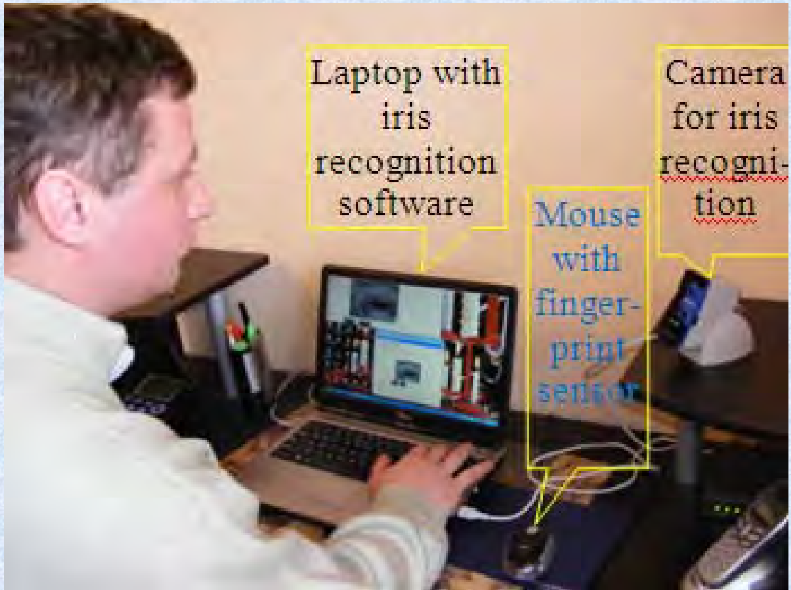
Multibiometric system, that consists of an iris recognition camera and a fingerprint sensor installed on a mouse
