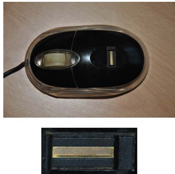
Figure 5. Mouse with a sweep fingerprint sensor and the detail of the sensor
