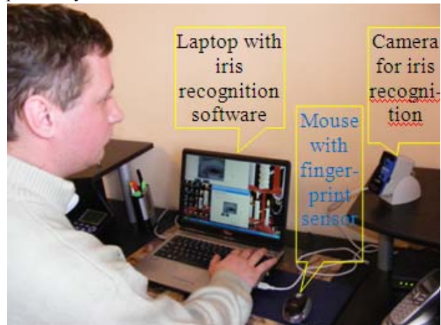
Figure 8. Multibiometric system, that consists of an iris recognition camera and a fingerprint sensor installed on a mouse
