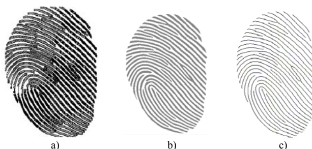
Figure 3. a) The image obtained after applying the Canny filters; b) image after smooting (filling gaps); c) image after thinning
