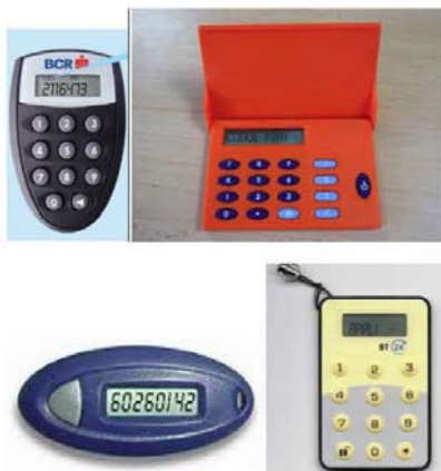
Fig. 2. Digipasses used for OTP generation (BCR, ING, OTP and Banca Transilvania)
