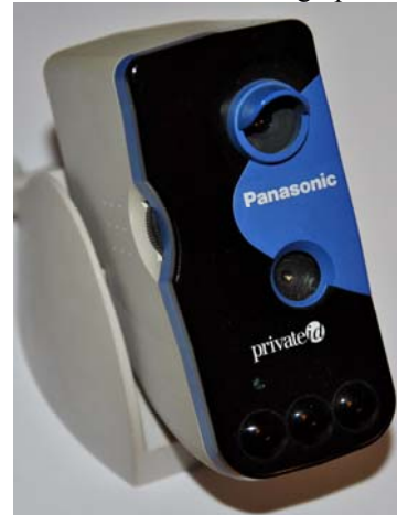
Fig. 8. Panasonic BM-ET100US iris camera and webcam
