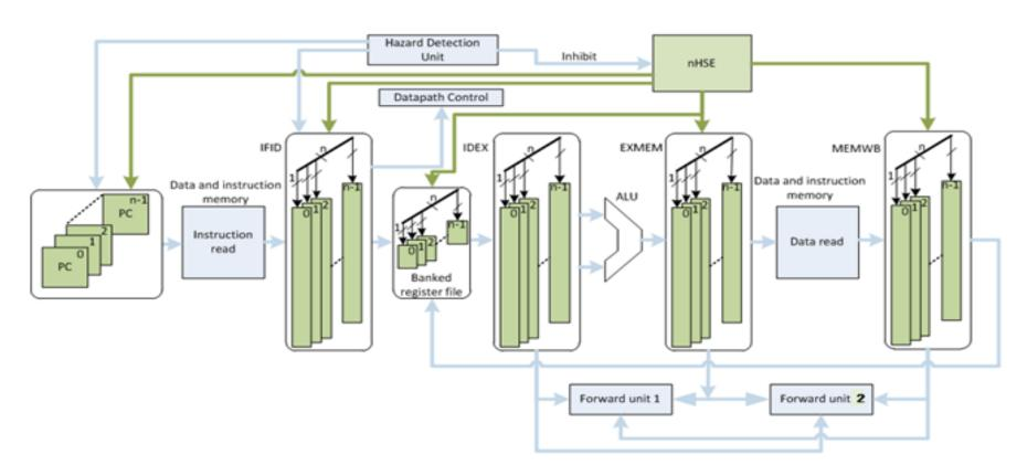
The context switching operations can be achieved in one processor cycle, and the response to an external event is delayed up to 1.5 processor cycles because each task has a set of pipeline.
